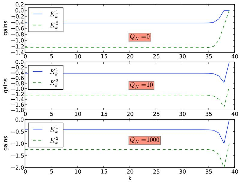
Figure 4.2: Controller gains  $K_k$  for different values of the final state cost matrix. Note in every case the rapid convergence as the horizon becomes more distant.
