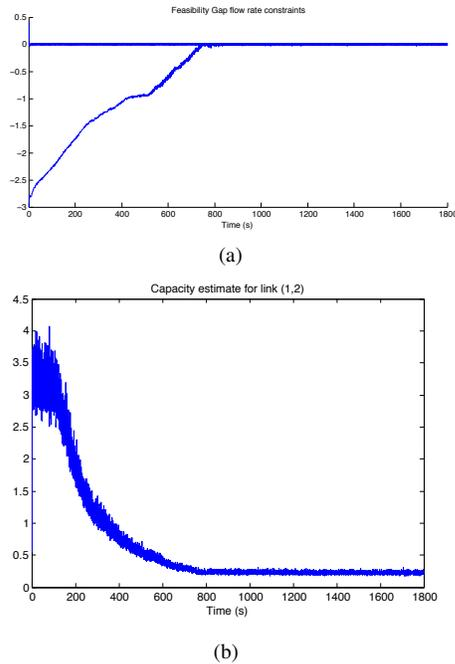
Fig. 3. (a) Trajectories of the routing constraint values  $g_i^\phi(a_i^\phi[k], r_i^\phi[k], r_i^\phi[k])$ . Note that the communication constraints are essentially always satisfied during deployment. (b) Sample trajectory of the capacity estimates (19) for the link (1, 2), with  $\gamma = 0.2$ .
