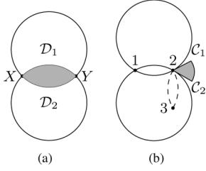
Fig. 1. A path between  $X$  and  $Y$  contained in the shaded region  $\mathcal{D}_1 \cap \mathcal{D}_2$  is called a direct path. On Fig. 1(b), the vehicle cannot pass through points 1, 2 and 3 using only direct paths. For direct paths  $1 \rightarrow 2$ , we show the range of possible final headings at 2, delimited by the tangent directions to  $C_1$  and  $C_2$ . We also delimit the region of direct paths  $2 \rightarrow 3$ .
