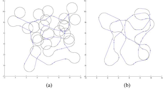
Fig. 4. Dubins tours through 50 points randomly distributed in a  $10 \times 10$  square. The turning radius of the vehicle is 1. (a) Alternating Algorithm (b) 10 discretization levels.
