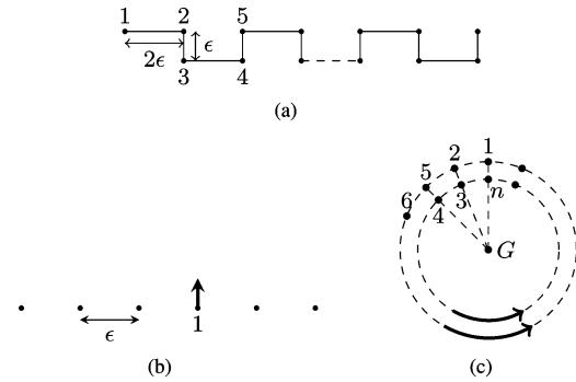
Fig. 2. Waypoint configurations that are hard instances for some proposed ordering methods. (a) ETSP ordering. (b) Nearest-neighbor heuristic. (c) Tang and Özgüner ordering.
