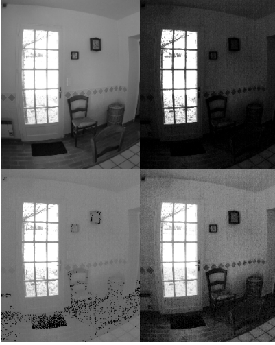
Figure 8: Mapping the lowest gain image to the highest gain image. (Upper Left) The highest gain image. (Upper Right) Estimating a model with only a multiplicative gain (Lower Left) A multiplicative factor and a bias. (Lower Right) Our Algorithm
