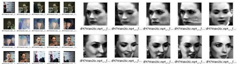
(a) A sequence of faces de- (b) The sequence after eye-pair filtering, alignment and cropping tected by the V. and Jones face detector
